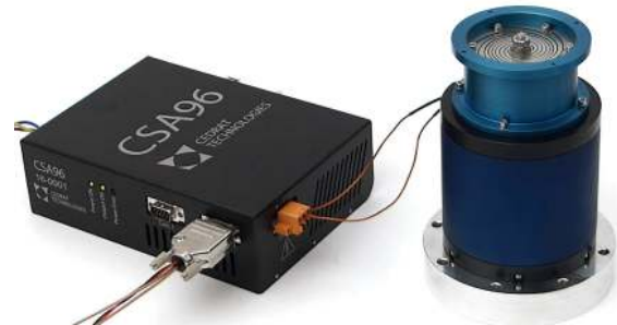
Fig. 6: MICA300CM Proof Mass prototype and CSA96
