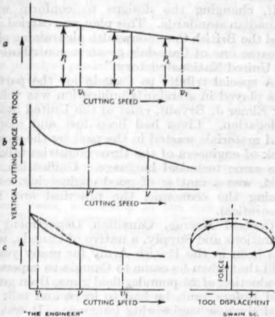
FIG. 7—Explanatory Diagrams of Cause of Self-Induced Vibration
