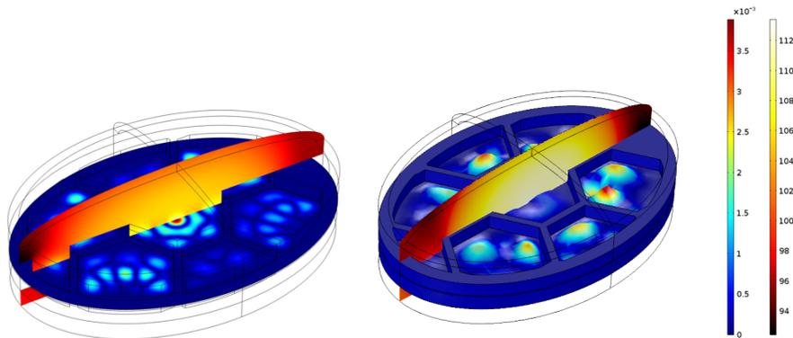
*Figure 2. Simulation plot showing the sound pressure level (thermal color surface) in dB and the displacement of the membrane (rainbow color surface) in mm from a fully coupled acoustics-MEMS model solved in the frequency domain. Left: solution at 5,000 Hz. Right: solution at 5,250 Hz.*
