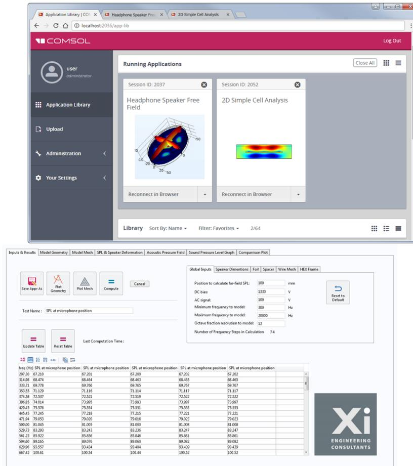
Figure 3. Bottom: The app developed by Xi Engineering allows engineers to vary parameters related to frequency, electrical input, speaker dimensions, and properties of the membrane, spacer, and wire mesh. Results give the sound pressure levels for different cases, membrane displacement, frequency response to different DC biases, and a comparison of the simulated design against experimental results. Top: The app is shared through the COMSOL Server™ product and accessible from a web browser.
