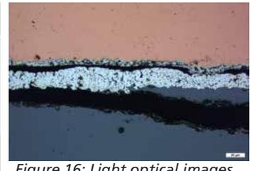
*Figure 16: Light optical images showing delamination of a contacted bus bar at the cell interconnect. Cracking can be seen across the wafer in dark gray at the bottom.*
