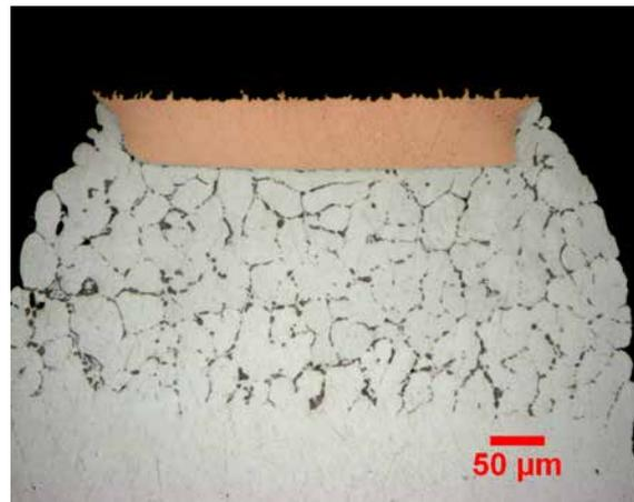
*Figure 10: Unetched SAC 305 Solder Alloy.*
