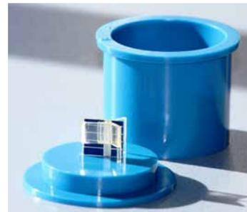
Figure 7: Solar cell with interconnector held perpendicular to the cross section with a UniClip Support Clip before epoxy mounting.
