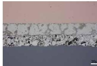
*Figure 17: Microstructure of Bismuth containing lead-free solder Sn60-Bi38- Ag02 (unetched) interconnect. Shown is the copper cell interconnect on top, bismuth solder layer, bus bar and silicon cell.*
