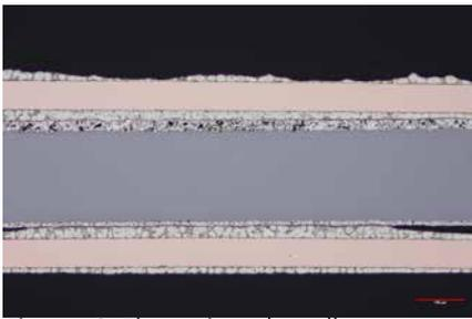
*Figure 13: The entire solar cells interconnect shows both the top and bottom soldered seams. The solder is not uniform and lacking at each end of the bottom seam.*
