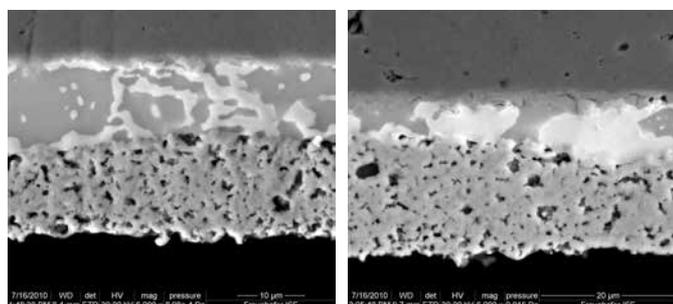
Figure 19: SEM image showing the intermetallic phase growth after accelerated aging. From the top, Silicon cell, (a.) Bismuth containing solder on (b.) bus bar.
