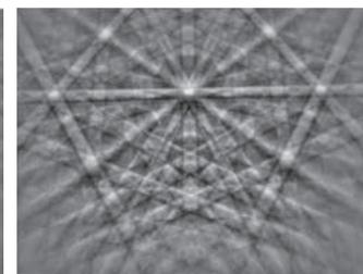
Figure 23: Standard Sample Preparation Plus Vibratory Polishing of Pure Single-Crystal, Band Contrast 233.
