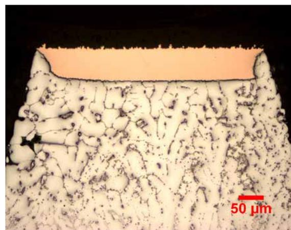
*Figure 11: Unetched SAC 305 Solder Photomicrograph after Vibratory Polishing.*
