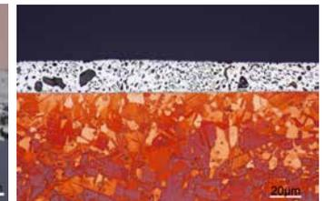
**Figure 18:** Sn62-Pb36-Ag02, etched with Klemm II, Eutectic solder material with Pb-rich solid solution (dark) and Sn-rich solid solution (light-colored). Annealing twins in copper (alpha solid solution).
