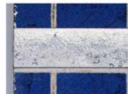
Figure 2: Interconnector on a soldered solar cell sample that exhibits a poor quality cut (top) vs a good quality cut.
