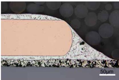
*Figure 14: Proper wetting angle of soldered copper*
