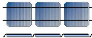
Figure 1: Solar cells connected in series with tabbing ribbons.
