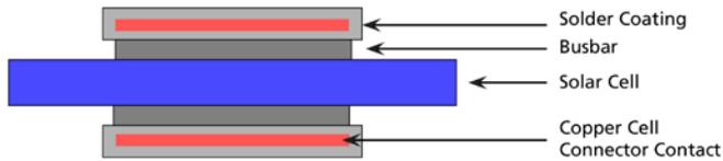
Figure 4: Drawing of a solder interconnect of a solar cell bus line.
