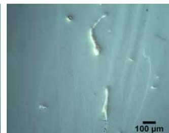
Figure 21: Polycrystalline silicon viewed with Nomarski DIC (etched: 100mL water, 75g NaOH)
