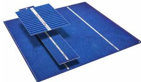
Figure 6: Sectioning the bus bar into samples appropriate for mounting. The first cut removes the bus bar trace. A second cut is made perpendicular to the bus bar section.
