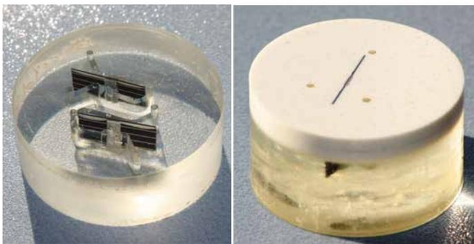
*Figure 8: Solar cell interconnects mounted in EpoxiCure® epoxy*
