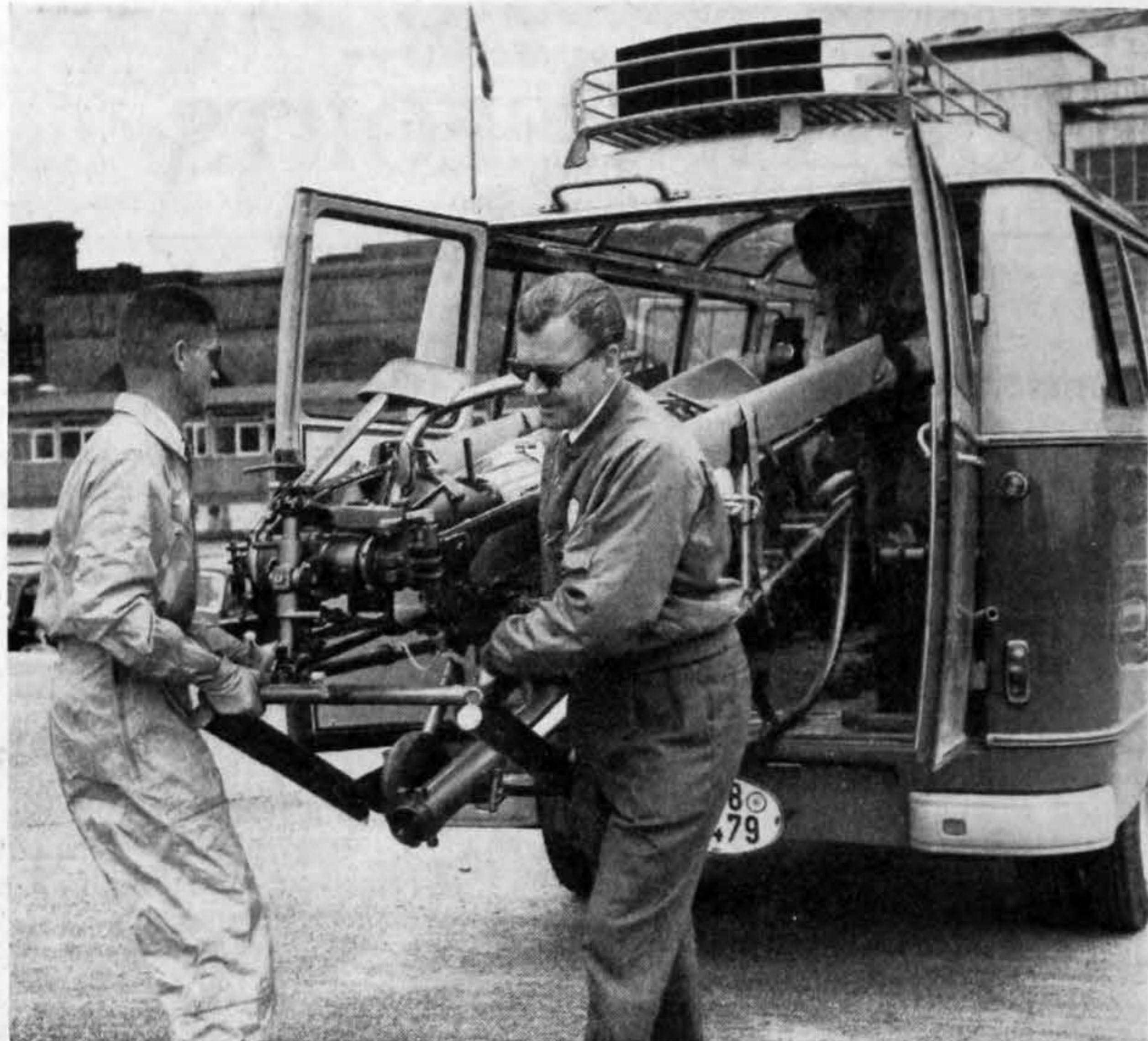
The machine is erected on a wheeled trolley. Notice the instrument panel, which is between the yaw control pedals; the pitot tube is supported directly off the air speed indicator
