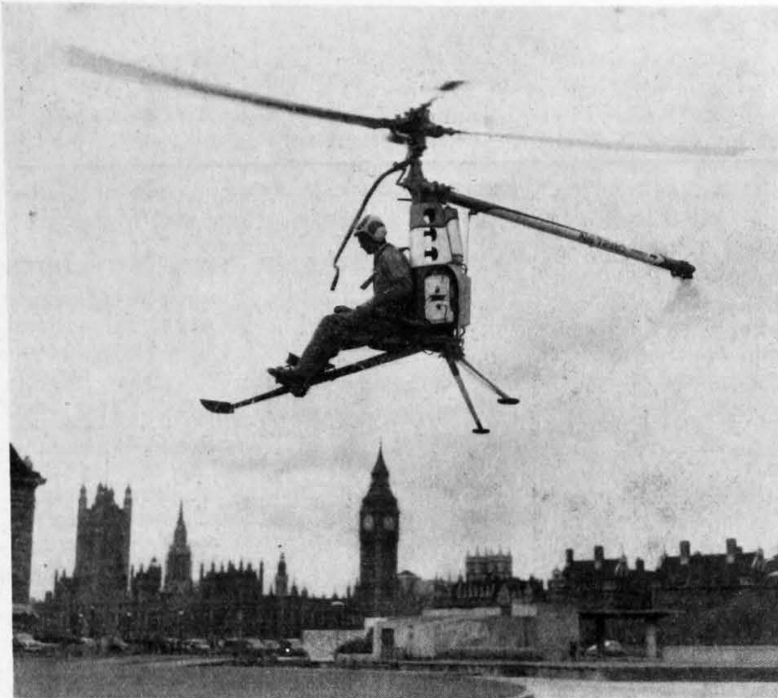
The "Rotorcycle" can hover without use of the cyclic pitch control during a demonstration. The holes in the sides of the "body" admit air to the horizontal cooling fan, which drives it over the engine
