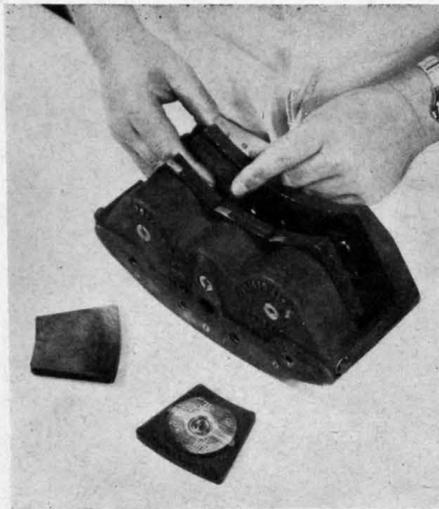
Friction pads are retained in the caliper by press studs: the pad is moulded to fit into the caliper or braking plate. Quick *in situ* replacement is not a requirement
