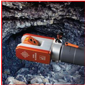
Deployed vertically or horizontally on a boom, Void Scanner can access hard-to-reach cavities.
