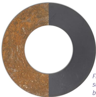
*Fig2: Corrosion and surface comparison between Polymer and Steel.*
