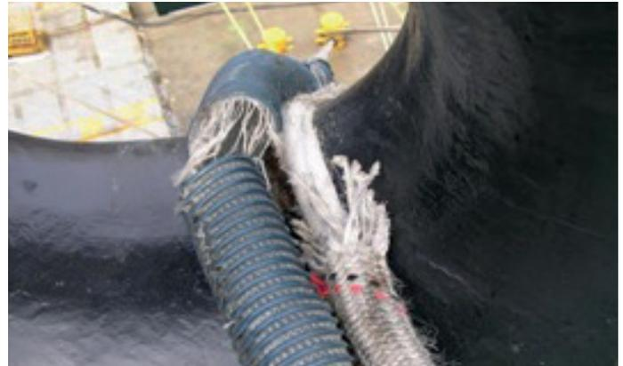
*Fig1: Wear sleeve, jacket and core damage.*
