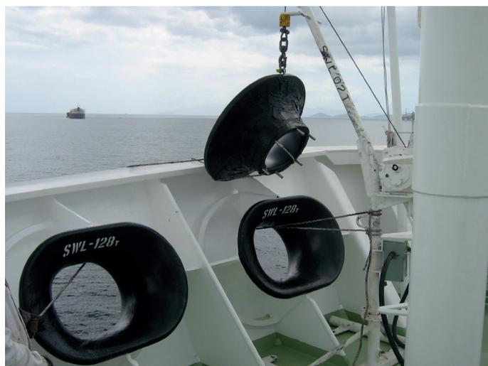
*Fig3: Chock Liner being fitted with standard equipment and no hot work.*
