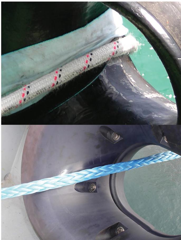
Fig4: Chock of moored vessel before (top) and after Chock Liner fitting (Bottom).
