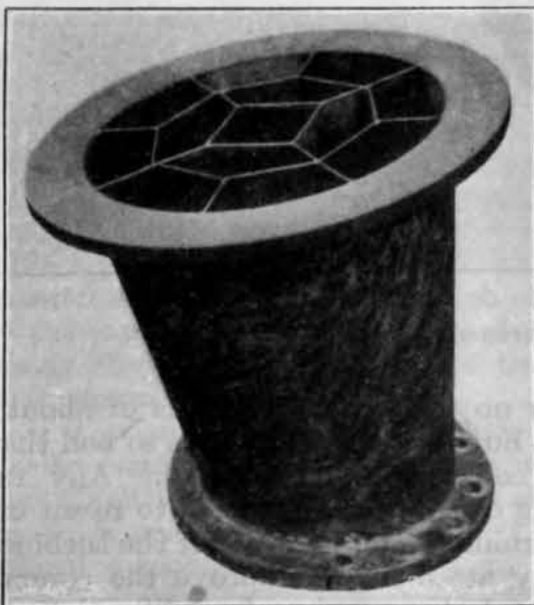
FIG. 9—The "Honeycomb" Diffuser used in the First Model of the Experimental Engine
