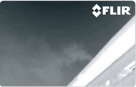
CO leak in off blast furnace
