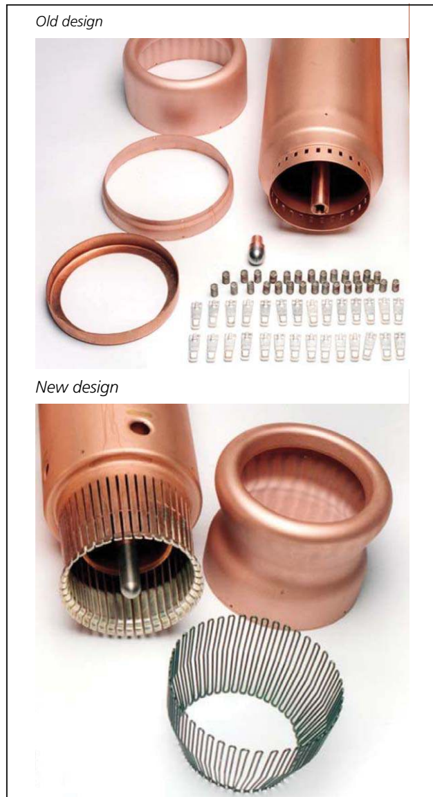
Example of simplified design. Current conducting parts of HV interrupter with integrated contact fingers
