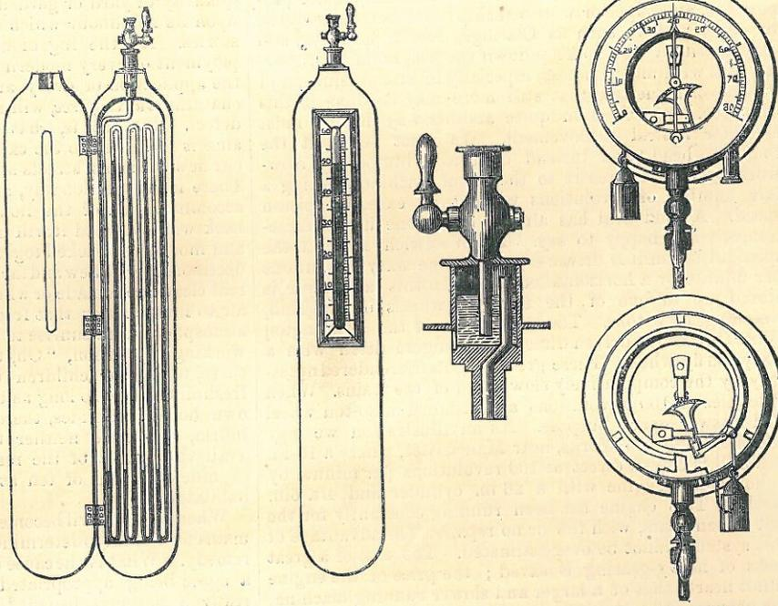
One of the principal features about the gauge is the tap on the top, which is so constructed that no dirt or water from the boiler can enter the first tube and come in contact with the mercury.
