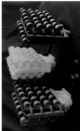
Example of disposable pattern, ceramic shell and casting
