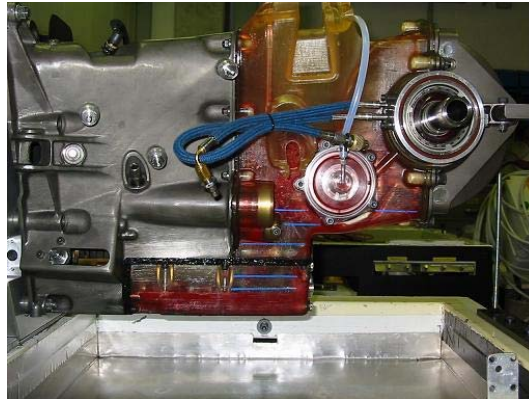
Figure 7: gearbox working (primary shaft rotation speed = 3,000 rpm) with 1.5 litres of oil inside
