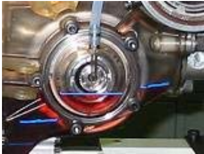
Figure 4: lubricating the bearings of the 3 rd shaft – zoom of the two side Plexiglas covers with the gearbox at a standstill
