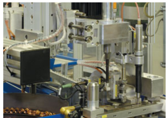
Automatic processing of HELICOIL® plus M 8 screwlock with vibration singling-out.
