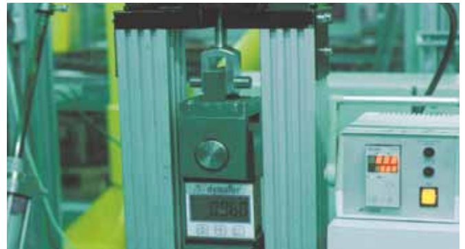
Test bench for loads up to 150 MPa and temperatures up to +250 °C
