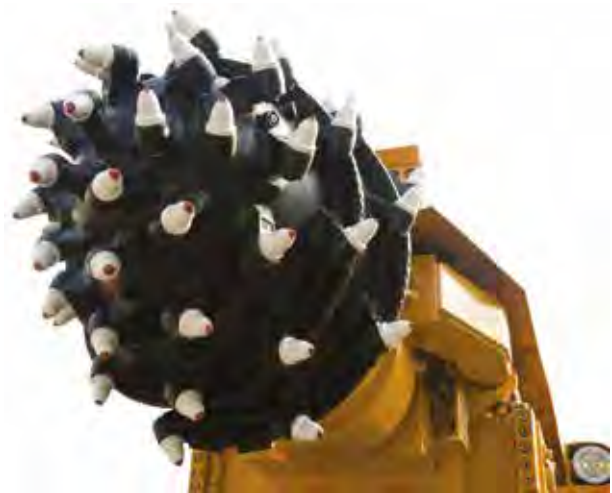
Road header cutter
