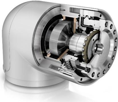
For the joints, Schaeffler offers a system assembly consisting of the DuraWave RTWH strain wave gear with the XZU angular contact needle roller bearing and the UPRS-series motor.
