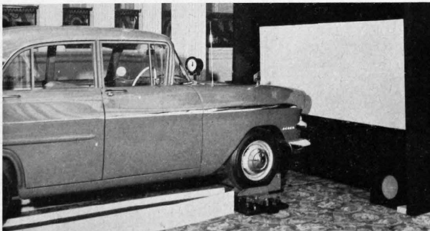
A "Victor" mounted on the simulator: the turntables supporting the front wheels can be seen. On the far side of the bonnet is a stop-clock displaying brake reaction time
