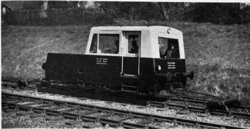
Matisa track recording trolley with outrigger detector assemblies extended
