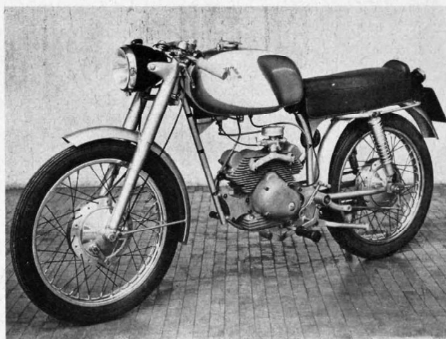
The 90 deg. V-twin engine of the "La Strada" has a single carburettor. In the lightness of the cycle parts the machine is typical of Italian design
