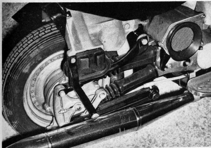
The "Berlin" is built extensively of light alloy
