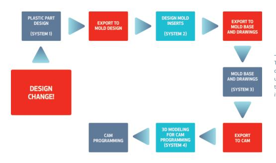
The nonintegrated approach to design-to-manufacturing adds unnecessary time and costs related to communication barriers and iterations late in the process.
