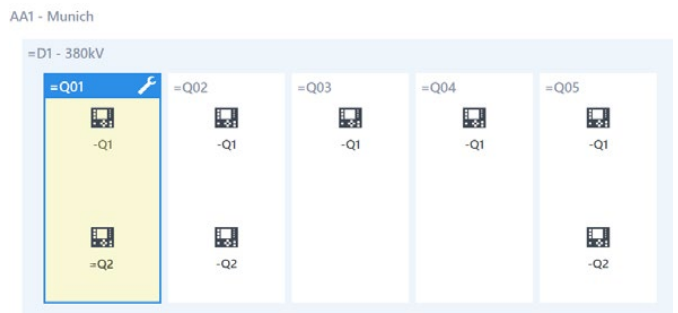
Figure 7: Maintenance mode activated for bay Q01.
