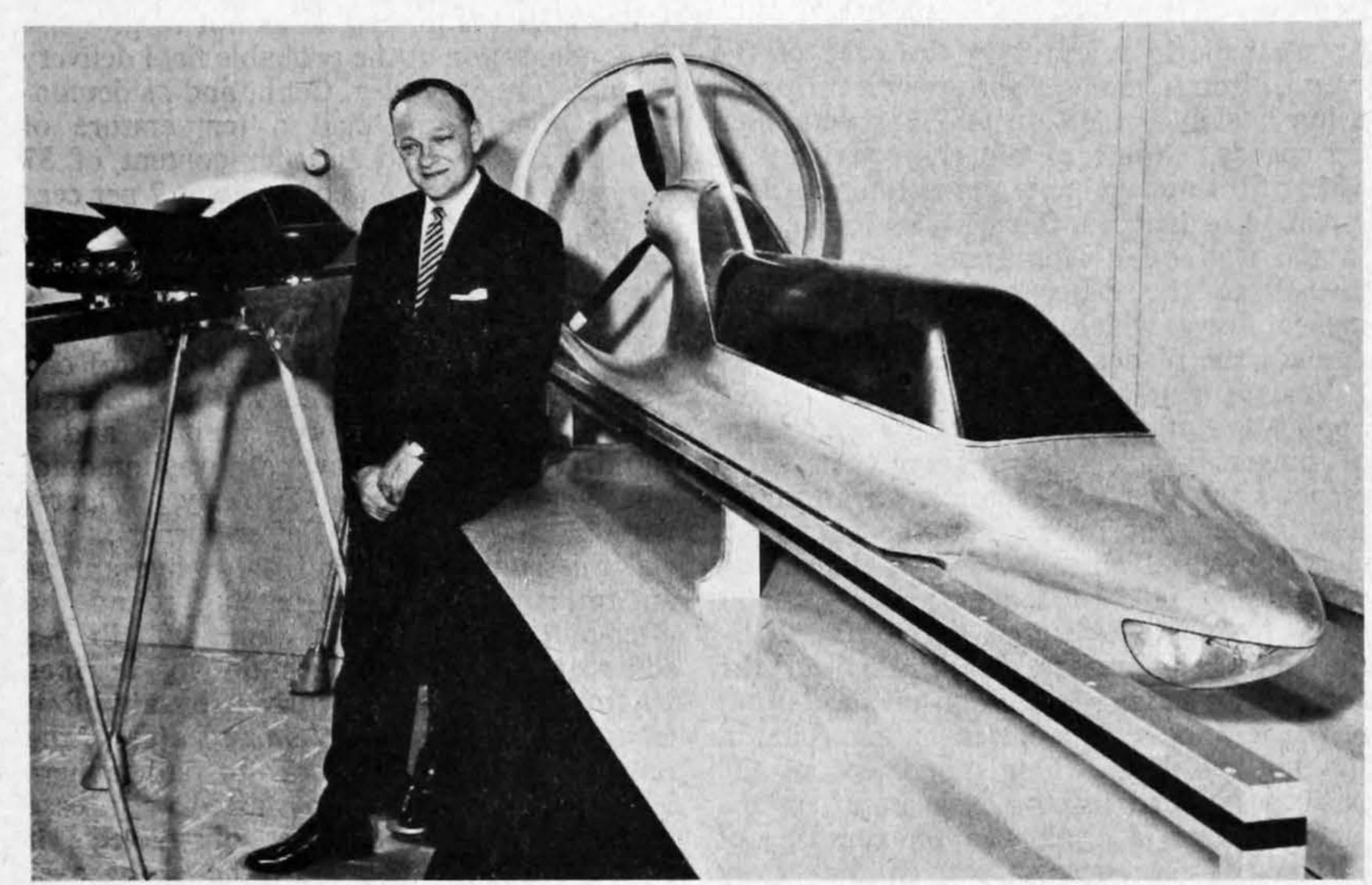
More than thirty years ago Andrew A. Kucher, now Vice President, Engineering and Research, Ford Motor Company, conceived the air-bearing vehicle, supported clear of its tracks by "levitation" on a thin film of air. The passage of a "Levacar" would be virtually frictionless, and while propulsion can be achieved with moderate efficiency at speeds of, say, 500 m.p.h. steering is not easily achieved to the standards of surface vehicles; hence it is anticipated that such vehicles would be rail-bound.
