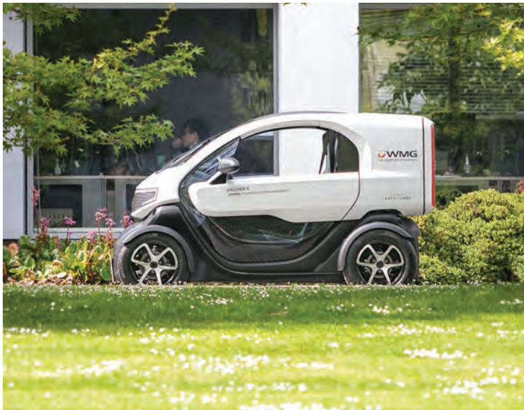
The demonstrator is based on the platform of the Renault Twizy
