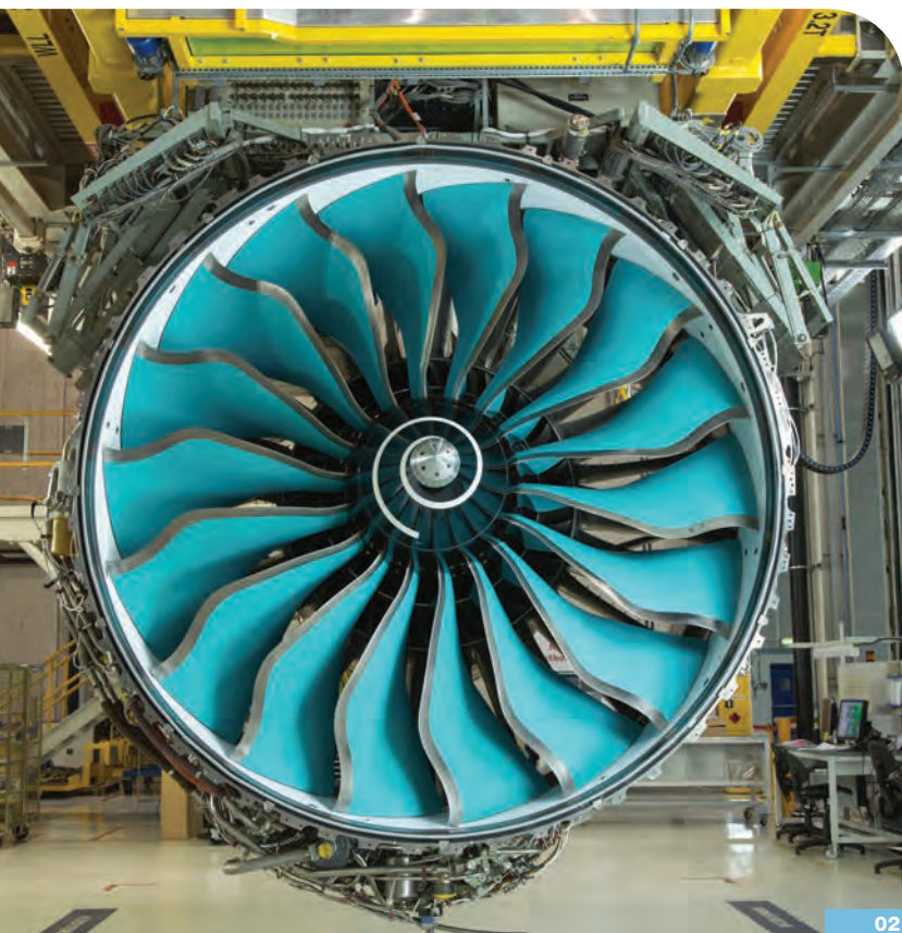
02 Rolls-Royce's Advance concept features carbon titanium blades
