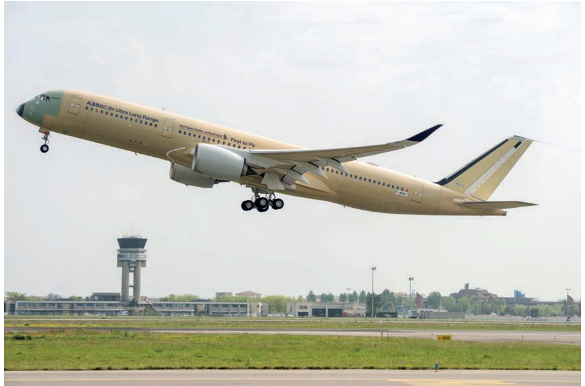
Airbus' new Ultra Long Range variant of its A350 aircraft has taken to the skies for the first time, ahead of entering service on the world's longest passenger route. The Ultra Long Range Airbus A350 XWB made a short maiden flight from Toulouse-Blagnac Airport as part of a test programme. The aircraft will have a range of 9,700 nautical miles.
