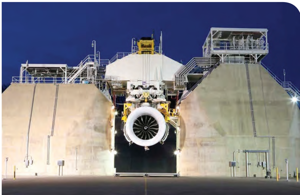
Ground tests have begun on the world's largest commercial aircraft engine. GE Aviation's GE9X is a 100,000-pound thrust-class engine that is going through its paces at the company's Peebles Test Operations facility in Ohio prior to initial deployment on Boeing's new 777X aircraft.
