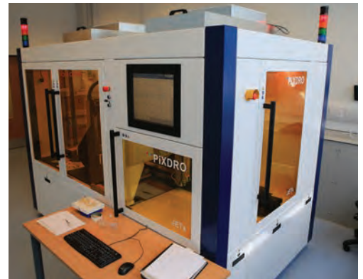
The Jetx3D can print different materials from each of its six heads
