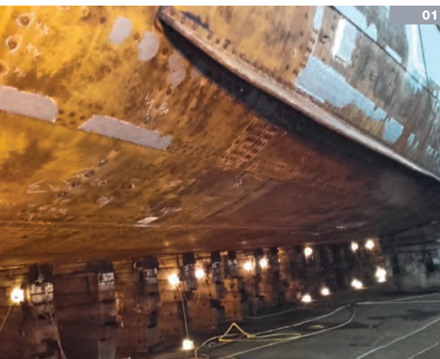
01/02 The century-old steel hull of HMS Caroline was badly pitted and would not withstand much welding 03/04 After applying the epoxy coating, the ship is now ready for the next phase in its long life
