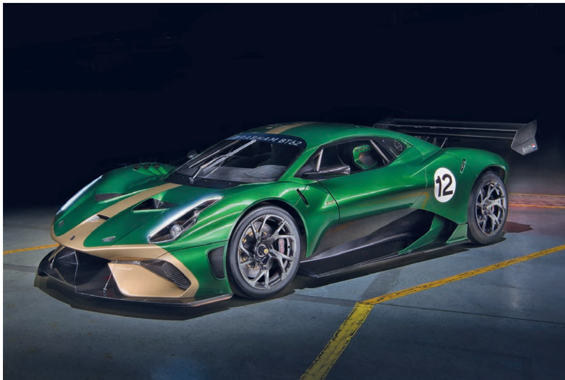
Brabham is back with the BT62, a £1m track-only hypercar that is set for a limited production run of 70 vehicles from facilities in South Australia. The BT62 is said to boast a power-to-weight ratio of 730ps per tonne, a dry weight of 972kg and is powered by a Brabham naturally aspirated 5.4 l capacity V8 engine.
