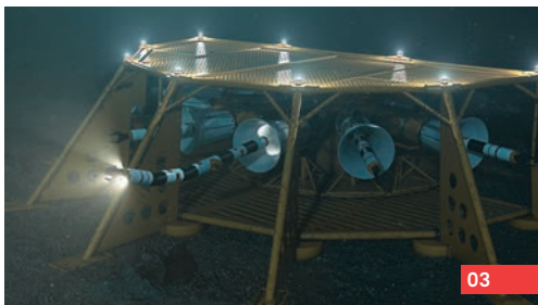
03 Eelume's underwater docking station for its inspection robots
