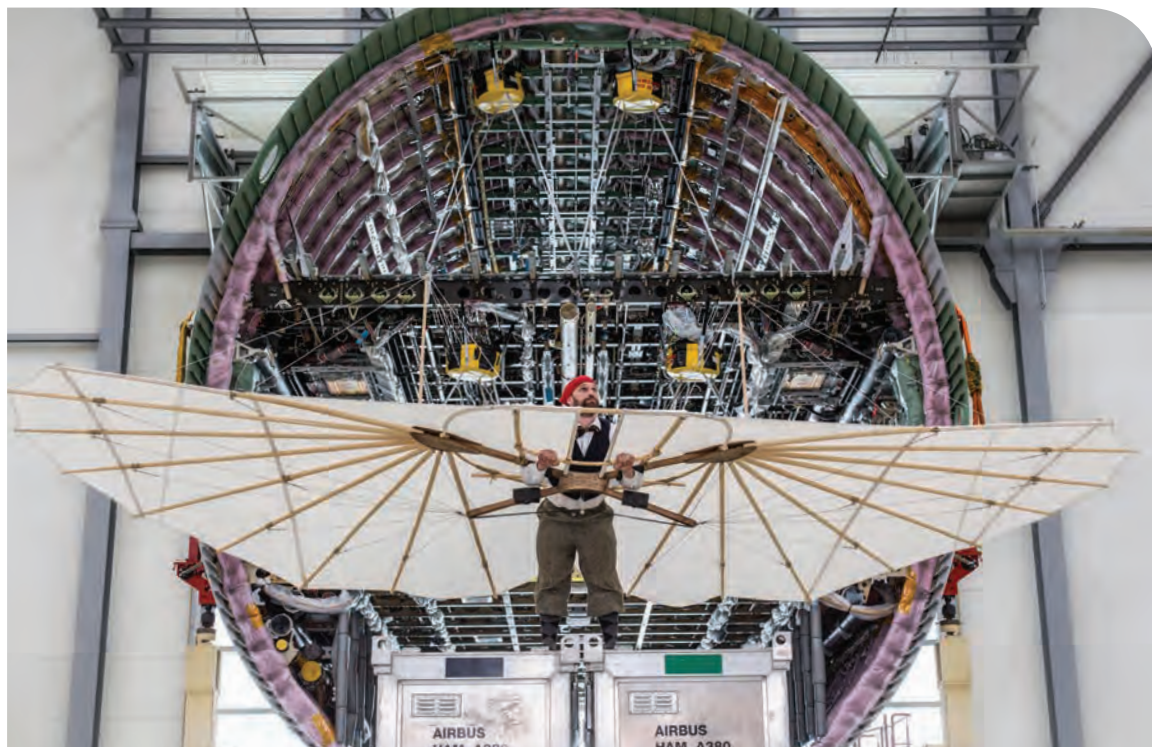
A lot has changed since Otto Lilienthal first took to the skies in Normalsegelapparat, the world's first series-built flying machine that has been replicated by the German Aerospace Center. Normalsegelapparat weighed 20kg and had a wingspan of 6.7m compared to the A380 it is pictured with, which has a wingspan of nearly 80m and weighs 569 tons.
