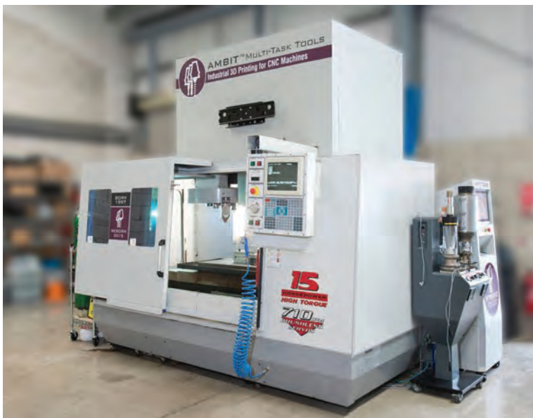
Hybrids system uses Beckhoff controls to integrate additive manufacturing with standard CNC machining
