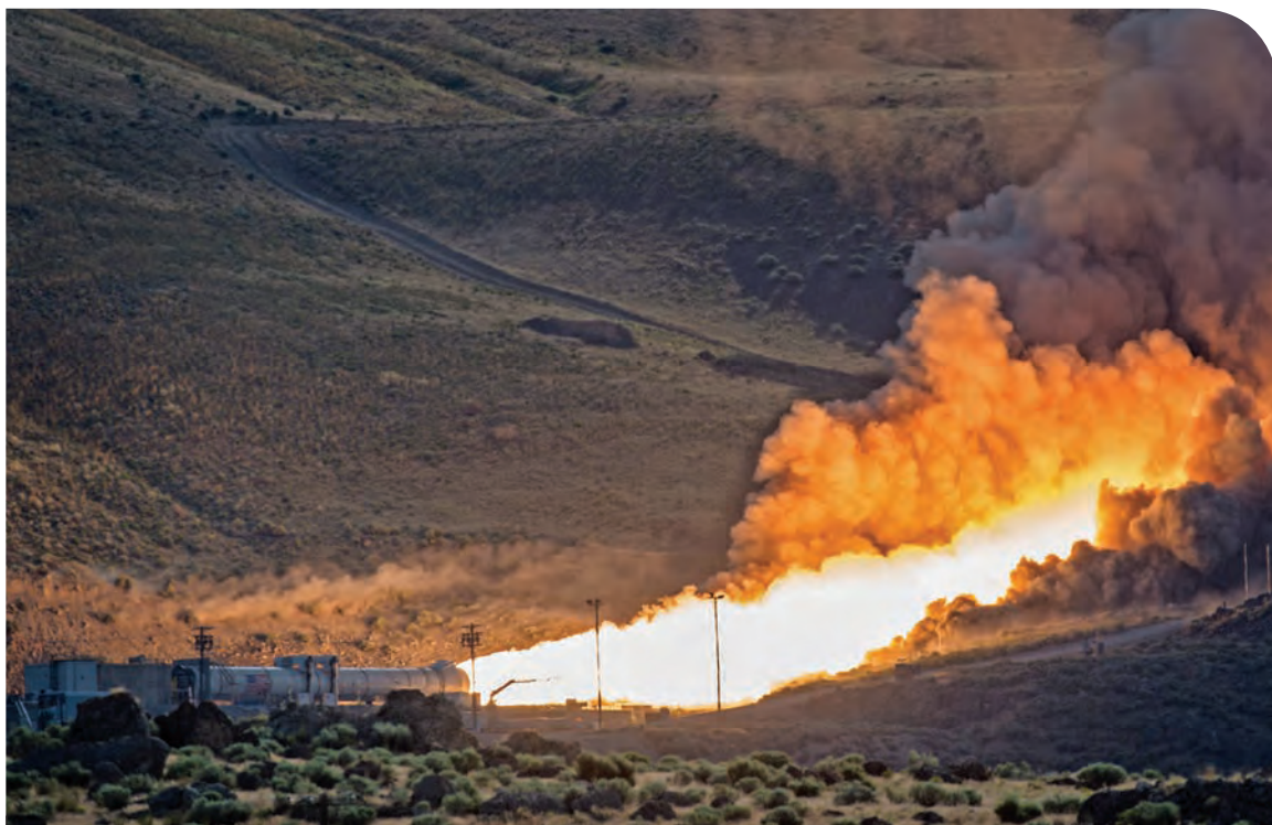
NASA's Space Launch System (SLS) has successfully fired up for its second qualification ground test at Orbital ATK's test facilities in Promontory, Utah. This was the last full-scale test for the booster before SLS's first uncrewed test flight with NASA's Orion spacecraft in late 2018.
