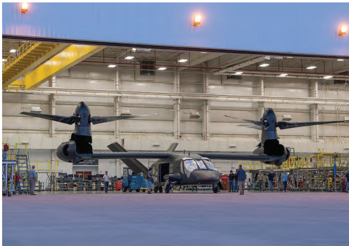
Bell Helicopter's V-280 Valor tiltrotor aircraft has made its maiden flight. The next-generation aircraft will be developed by a team that includes GE, Lockheed Martin and Moog. It will have a speed of 280kt and a combat range of 500–800nm.
