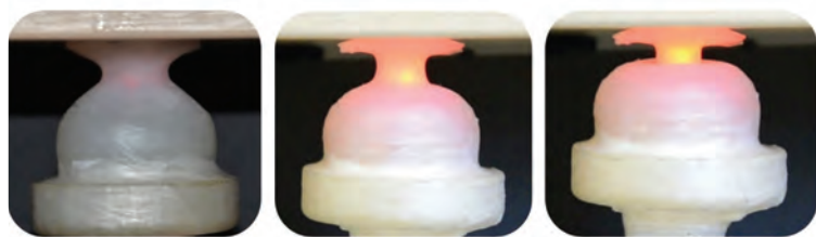
The Royal College of Art's sensorised mechanism acts as an anchoring module
