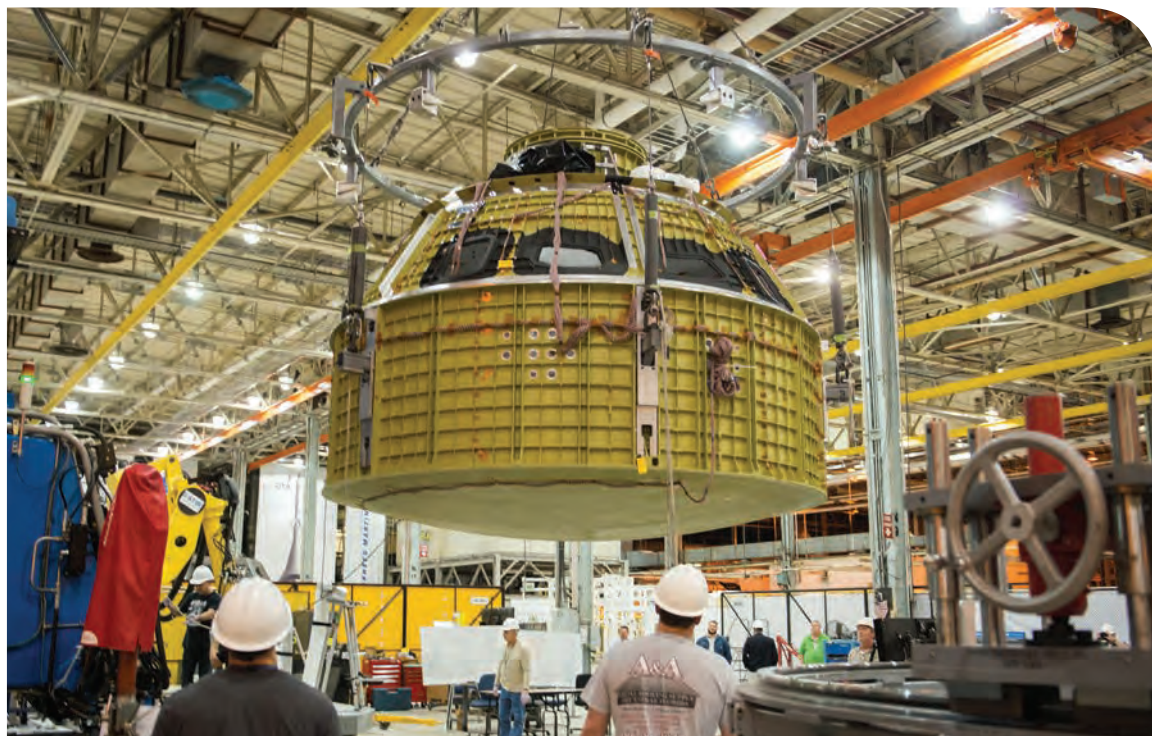
In January 2016, technicians at NASA's Michoud Assembly Facility in New Orleans finished friction-stir welding the primary structure of the Orion spacecraft, which is set for a deep-space mission aimed at informing the agency's target of reaching Mars.
