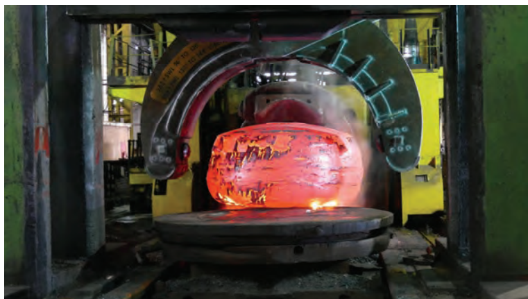
Forging the trial reactor pressure vessel head
