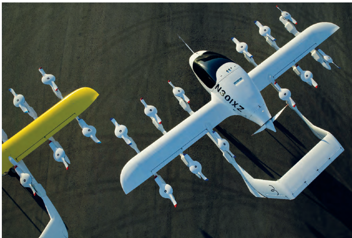
An electric air taxi that can take off vertically and fly autonomously has been undergoing testing in New Zealand. Dubbed Cora, the prototype two-seater aircraft has been developed by Kitty Hawk, a Silicon Valley-based aviation start-up. The aircraft takes off using 12 independent lift fans and is powered in fixed-wing flight by a single propeller.
