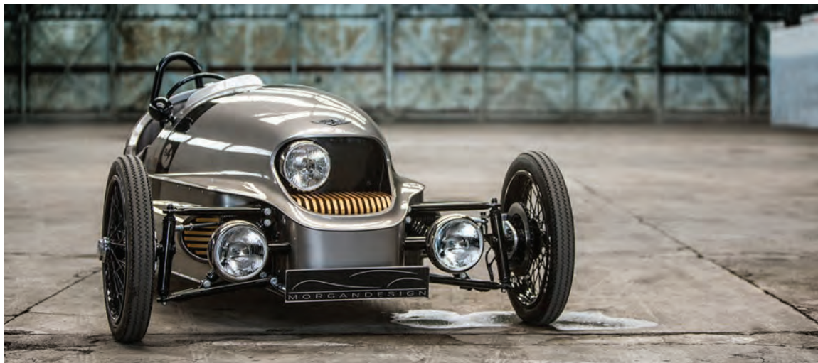
The EV3 has seen the use of carbon-fibre body panels for the first time in a Morgan car
