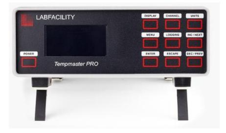
The Tempmaster PRO provides precise Platinum Resistance Thermometer temperature measurement and logging for exacting applications in both laboratory and site locations. It is an exceptionally accurate and stable digital thermometer particularly suitable for use with thermal calibration baths as a reference standard.
