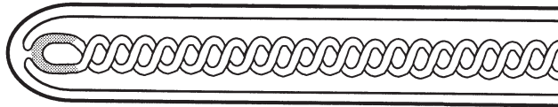
Fig 10: Fabricated Thermocouple Insulated, Twisted Pair Thermocouple inside Stainless Steel Sheath. Measuring junction earthed in this example.
