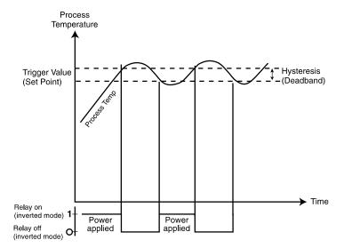
With On-Off temperature control, the output from the instrument is either on or off; the output is switched from one state to the other when the process temperature goes above or below the set point (trigger value). For the control of heating, the output is 'on' when the temperature is below the trigger value and 'off' when it is above the trigger value.
