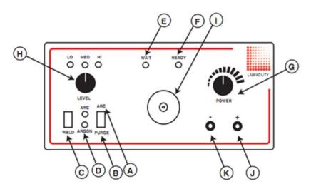
**A – ARC:** Argon gas and weld current controlled by the "Weld" switch. LED indication.
