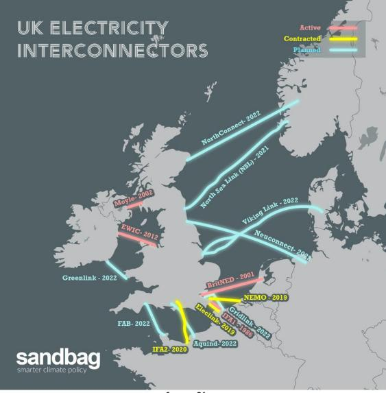
Figure 8. Active, contracted and planned UK interconnectors
