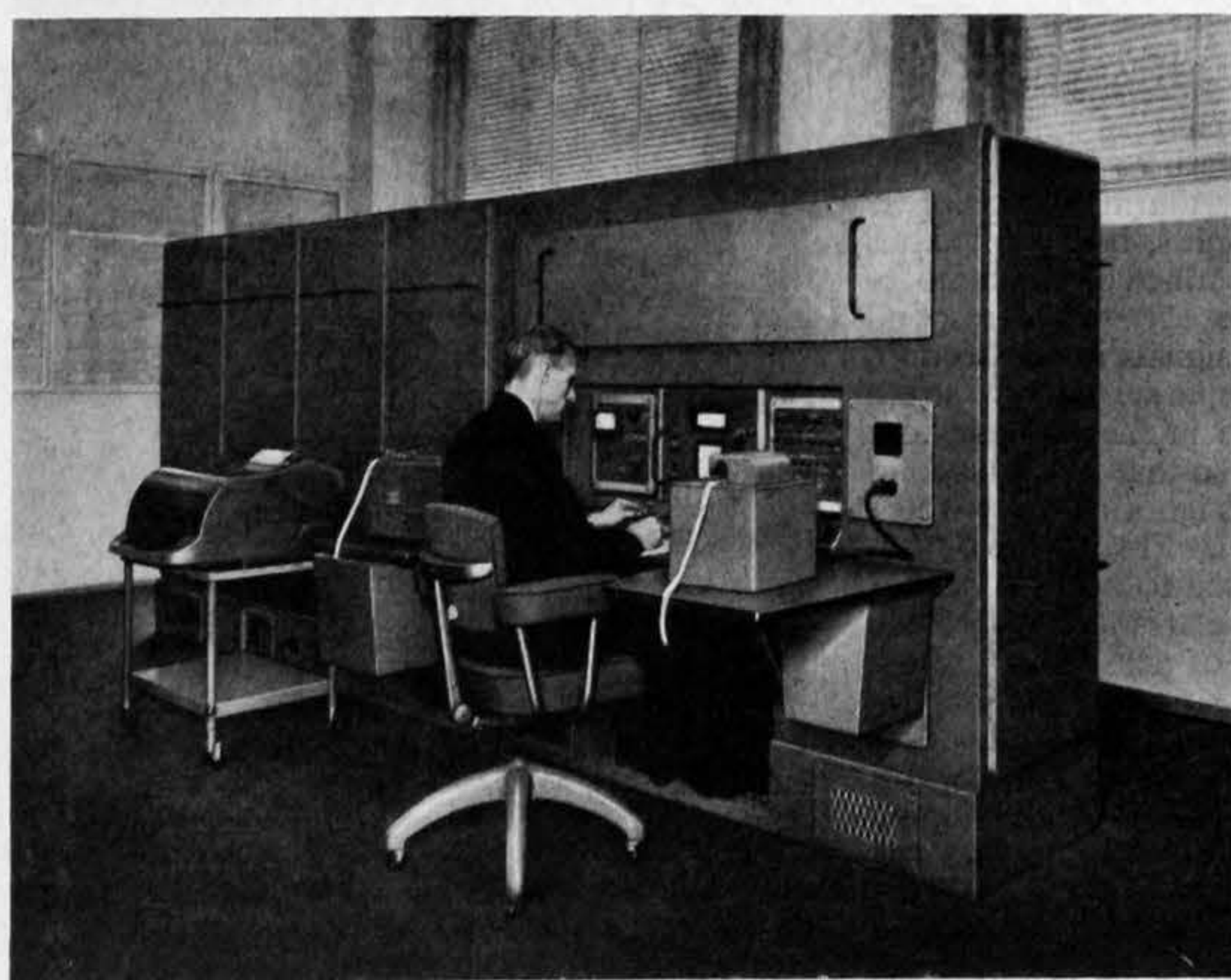
"Metrovick 950" digital computer. Most of the circuits consist of plug-in boards with printed wiring and transistors instead of thermionic valves. (Right) The magnetic drum of the computer. One of the four sets of read/write heads is in position in front of the drum. Another set has been removed from the left to show the drum surface
