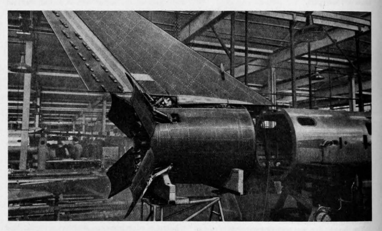
Fig. 2-Rear fuselage, showing dive brakes extended and fuselage break
