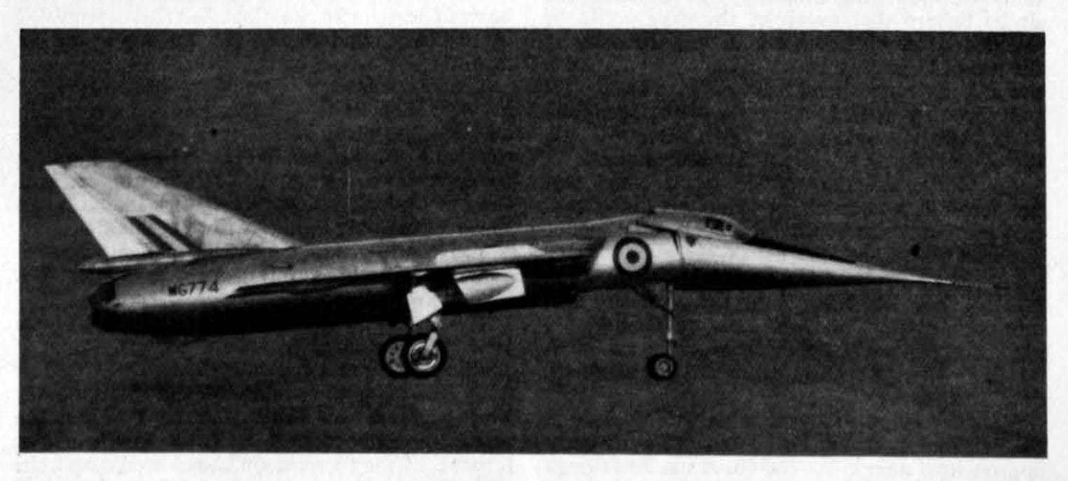
Fig. 1-Aircraft with nose drooped
