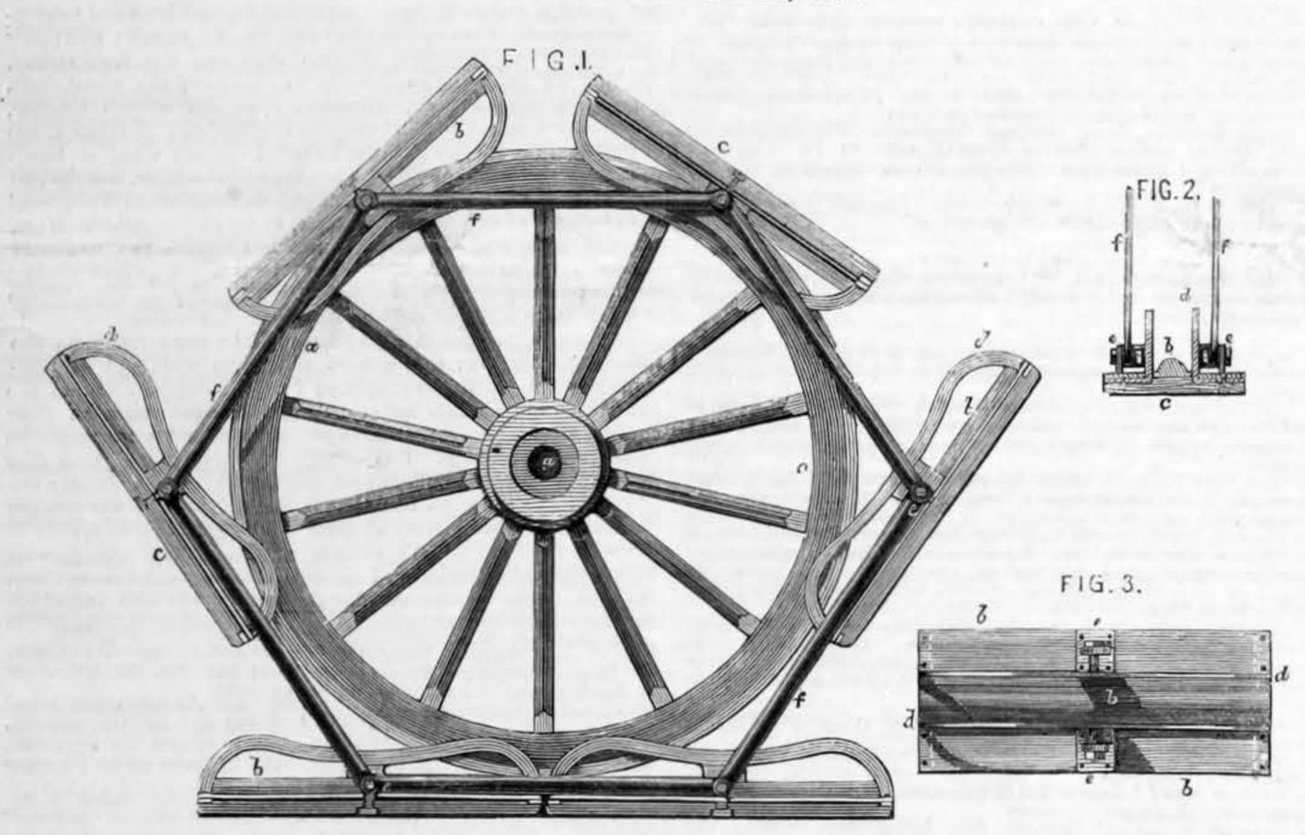
This invention consists in a new mode of constructing portable or endless railways to be applied to the wheels of engines and carriages, for the purpose of facilitating their movement over loose ground and irregular surfaces.
