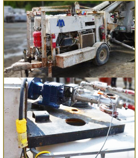
Shotcrete pump and accelerator pump
