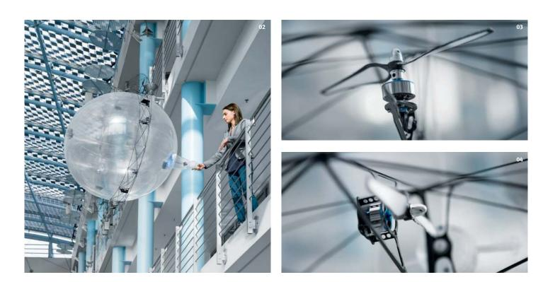
The propellers on the FreeMotionHandling are no longer located directly on the ball, unlike the eMotionSpheres. Just like the entire onboard electronics, the eight adaptive drives are fitted on the ultralight flying ring, which could thus also be used without the helium ball.
