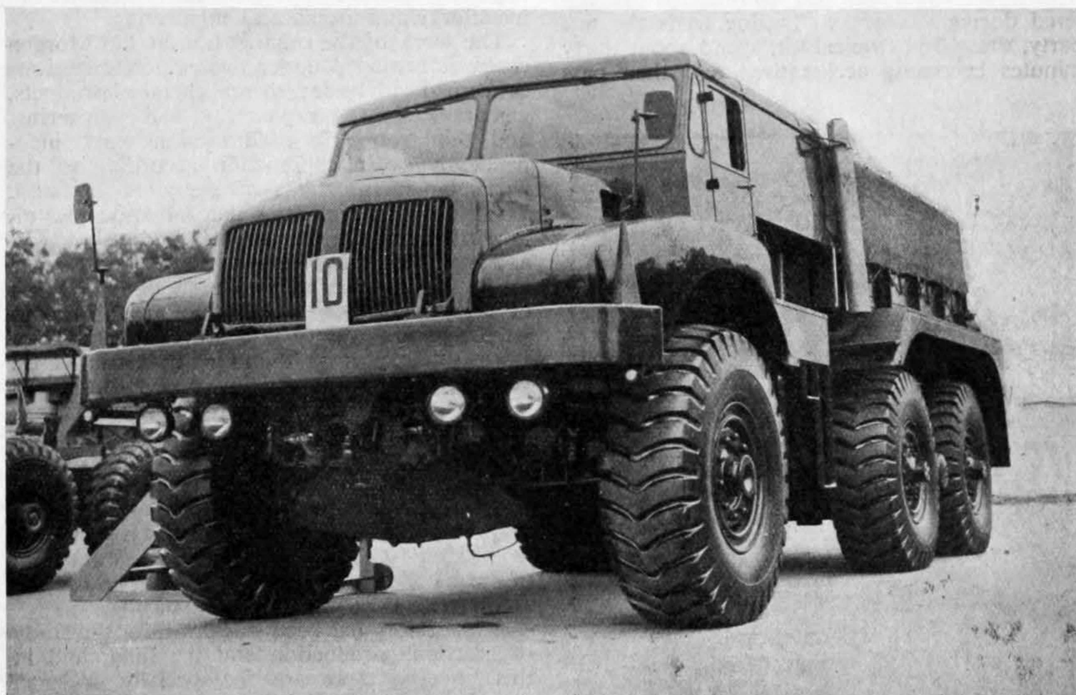
30-ton heavy artillery tractor. The articulated subframe, giving 2ft of wheel travel, can be seen and, dangling below the axle, one of the air pressure and temperature instrumentation leads. The outrigger bearing for the walking beam appears between the rear wheels
