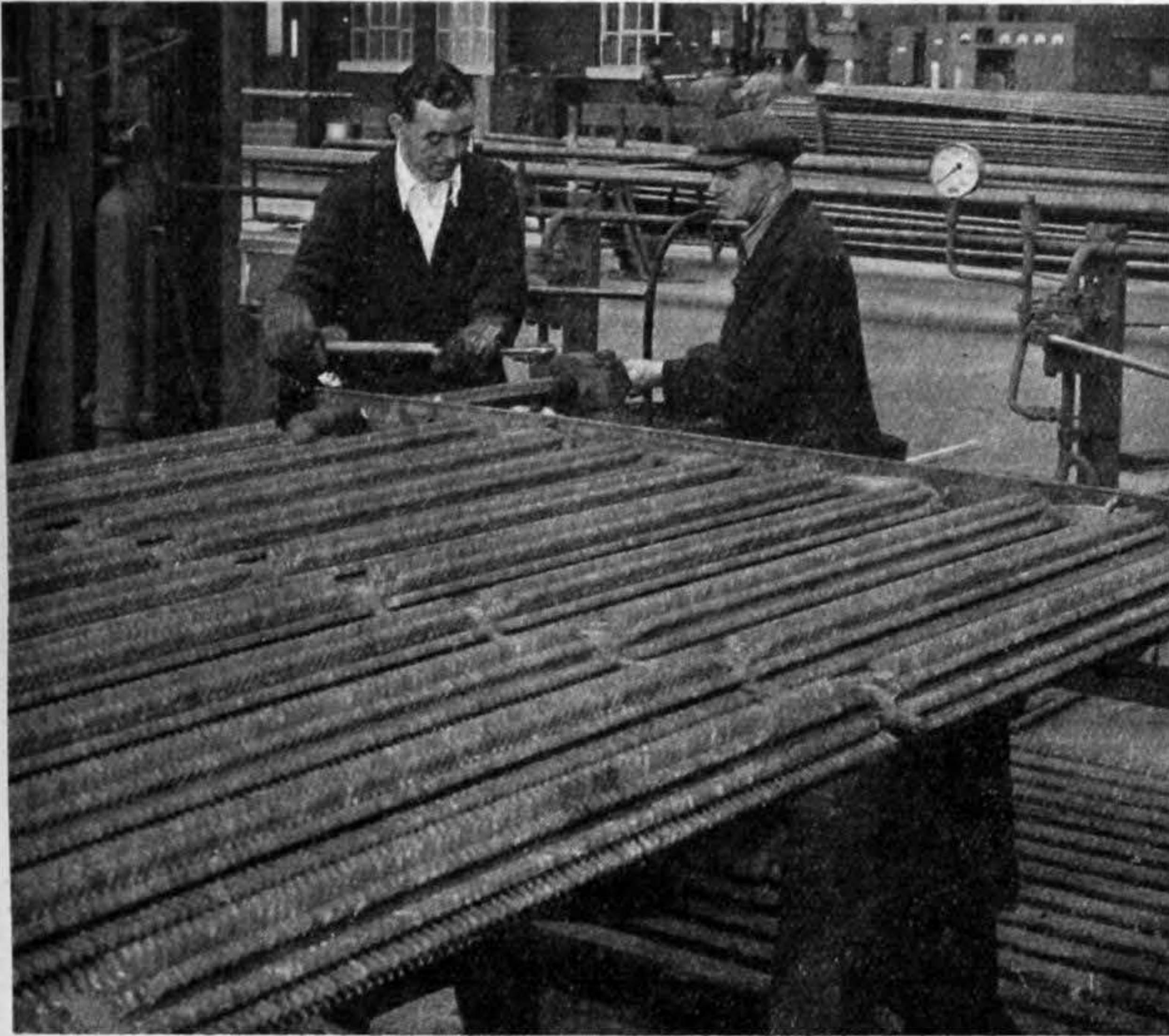
Fig. 11—Finned tube element for a heat exchange section undergoing hydraulic test in the workshop
