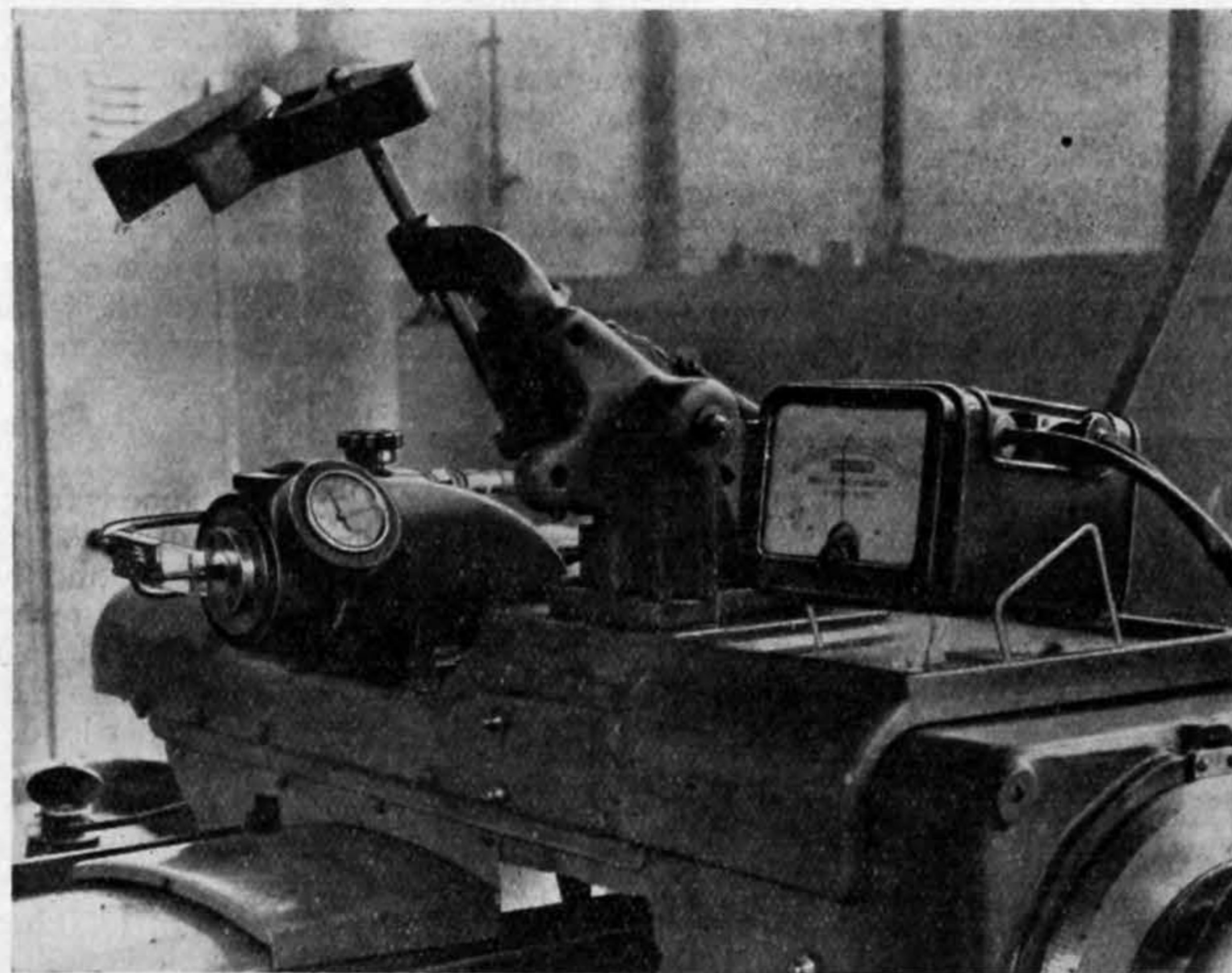
Internal grinding machine fitted with hydraulically driven grinding spindle and electronic tachometer
