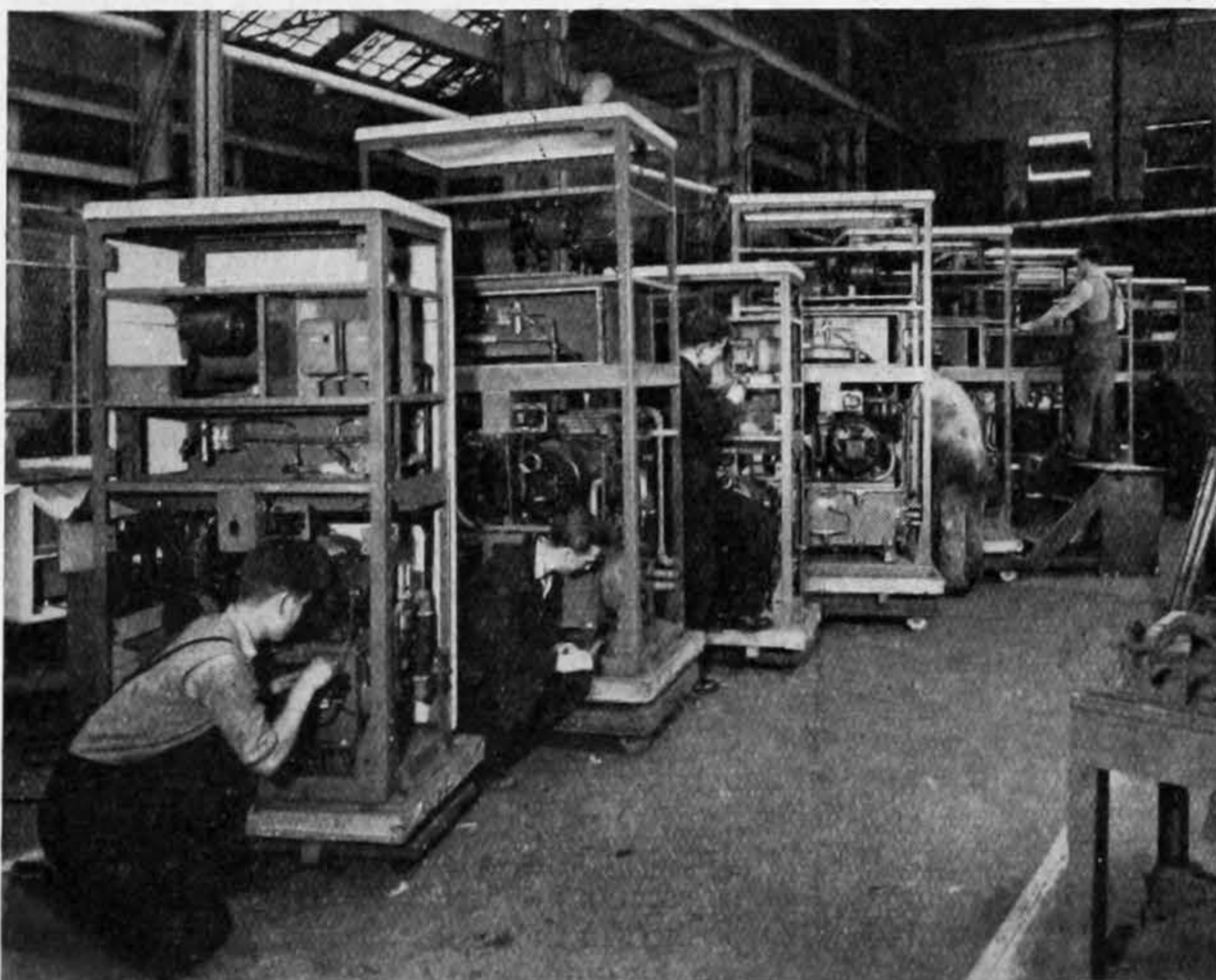
Type "S" thermo-units being assembled
