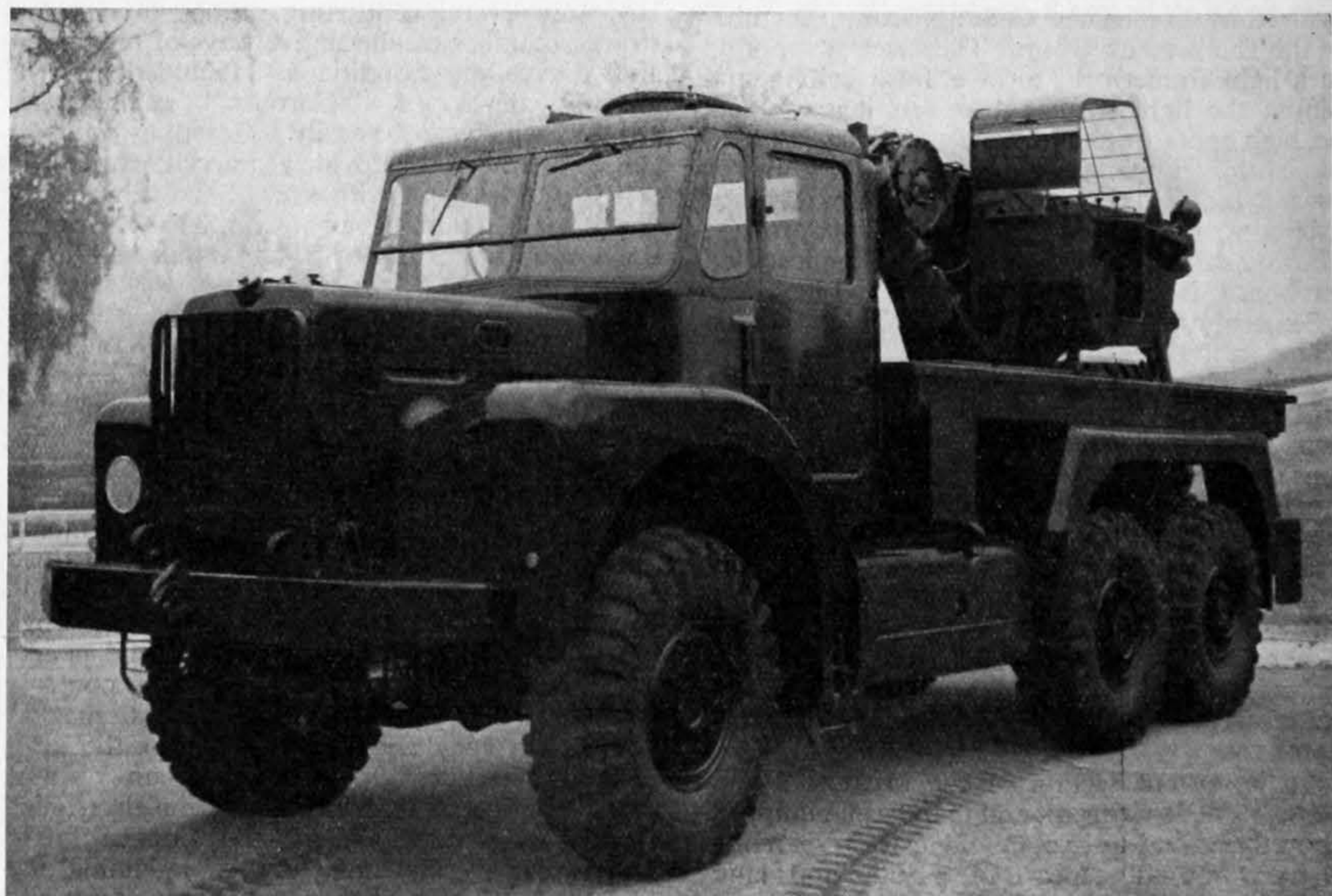
Heavy recovery tractor, showing the hydraulic motor, driving the crane hoist drum and the crane operator's cab
